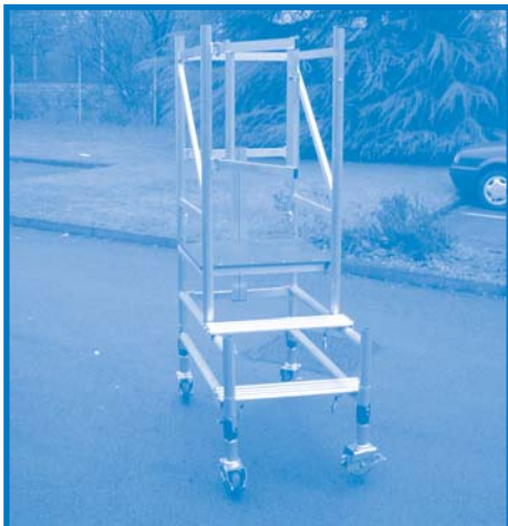
4. Locate the platform unit onto one of the three lowest rungs of the two end frames.
